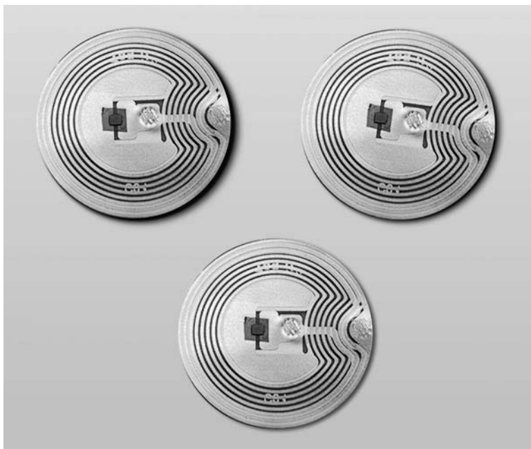
Figure 3-6 13.56-MHz Tag-It inlay (Source: Reprinted by permission of Texas Instruments Incorporated).
