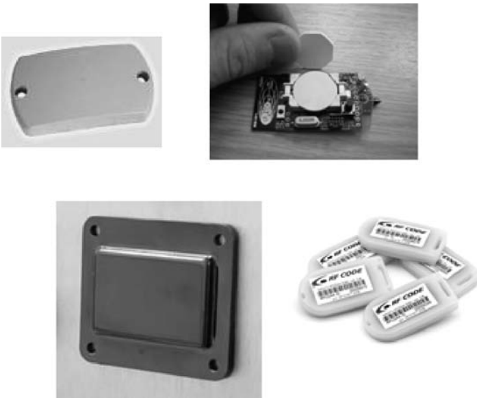
Figure 1-6 Active RFID tags (Courtesy of RF-Code, Inc.).
